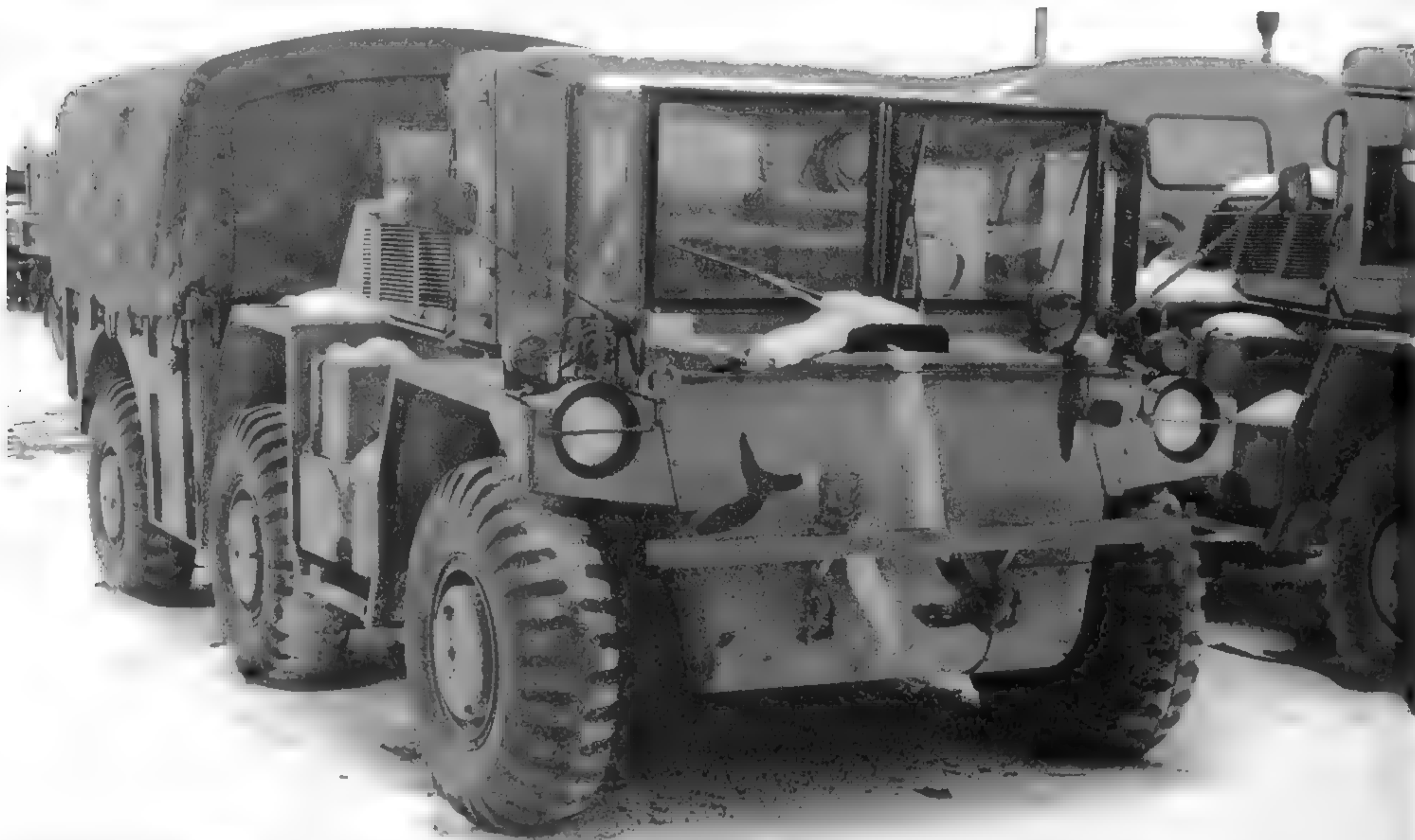
Many of the Gama Goats received the four-color MERDC paint scheme. This truck has a soft top, but all the top panels are installed, totally enclosing the cab. (U.S. Army photo)
